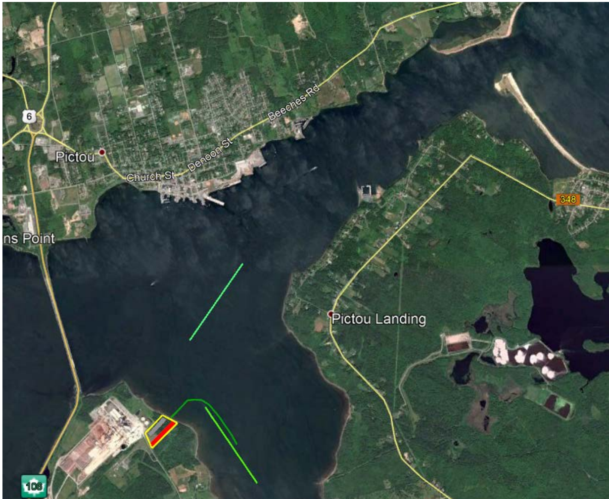
Figure 9. Schematic of primary staging site (yellow box) with pipe sticks (red lines in staging site), pipe weight storage (gray area in staging site), and the initial floating and towing stages for longer pipe lengths from Pictou to Caribou Harbor (green lines representing initial deployment, tow hookup, and towing).
