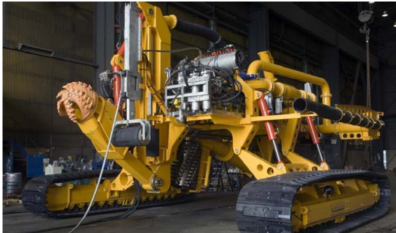
Figure 21. Mechanical Subsea Pipeline Trenching Machine, showing the rotating cutting head used to break through stiff soils or rock.
