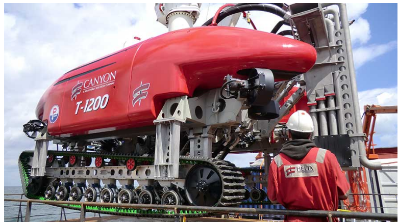
Figure 20. Water jet trenching / burial ROV
