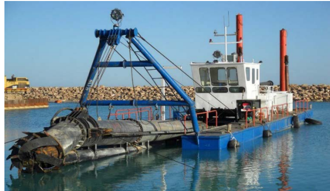
Figure 17. Cutting Suction Dredge
