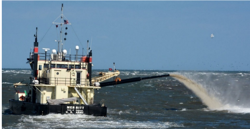
Figure 18. Side cast Dredge Merritt, Corps of Engineers
